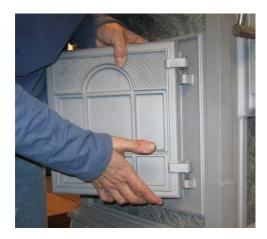
3. Place the door face down on a suitable work surface. Spray the set screw (on the side of the latch) with penetrating liquid to help loosen it. Do not spray liquid on the door stone (Keystone) as it may cause staining.
