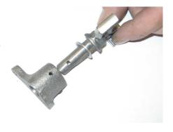
6. The new knob and latch have been pre-drilled, as a pair, to accept a roll pin, which will lock the two pieces together. Turn the knob to the full open position to expose the roll pin hole. Insert one end of the roll pin into the hole and carefully tap it through the assembly until the end of the roll pin closest to you is flush with the outside surface of the latch. (The flat spot in the knob should face the bottom of the door.)
