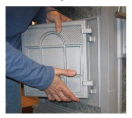
8. If necessary, adjust the tension on the door by manipulating the latch adjustment screw and lock nut. Turn the screw clockwise for more tension and counter clockwise for less. Tighten the nut to lock it in place.
