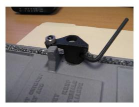
5. Place the shim from the old knob onto the shaft of the new knob and place knob in the door. The latch adjustment screw and lock nut should be at the top and against the stop on the inside of the door.
